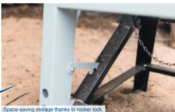
The indents in the rocker prevent the round material from slipping through
