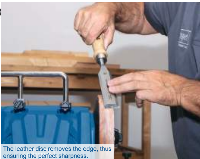
Shatterproof water tank prevents annealing of the blade.
