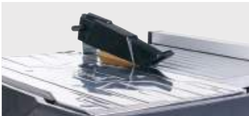
180 mm Ø diamond cutting wheel
