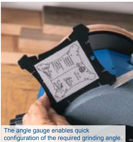
Grinds axes up to 170 mm head length.
